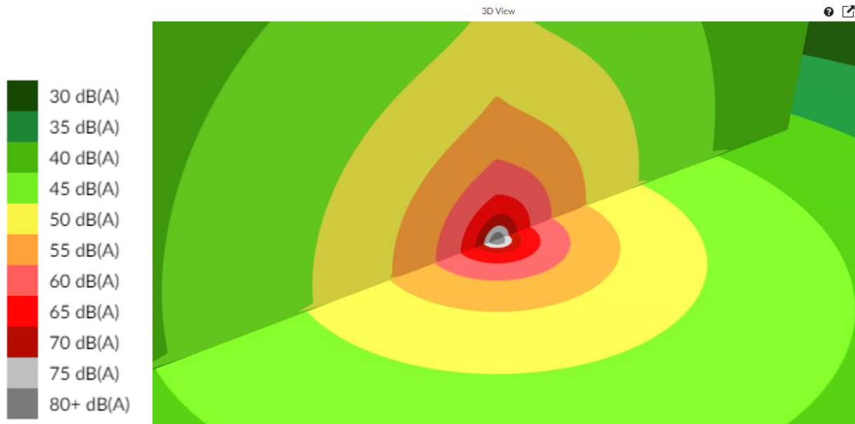
Figure 4 – Sound propagating away from a point source in a horizontal and vertical plane
