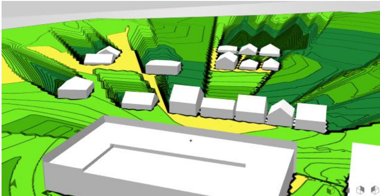
Figure 13 – Noise levels in OWAN from court 3 with 10 foot sound barrier – 3D view
