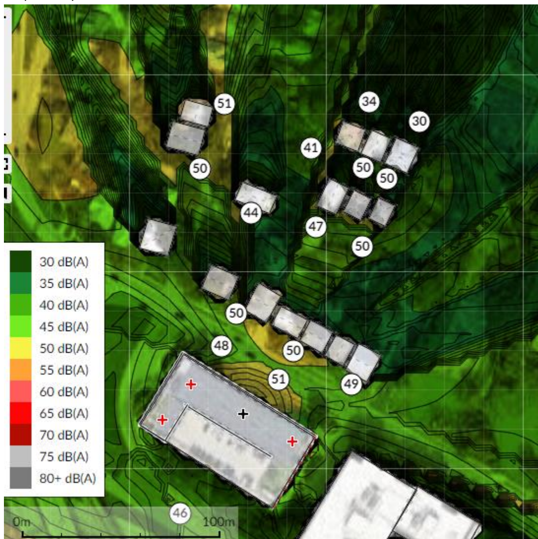
Figure 11a – Noise levels in OWAN from court 3 with 10 foot sound barrier on northeast and northwest perimeter
