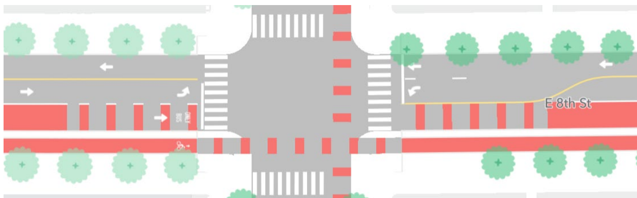
Figure 2 - Two-way street configuration featuring a transit-only lane and bicycle facility at an intersection with a dedicated left-turn lane
