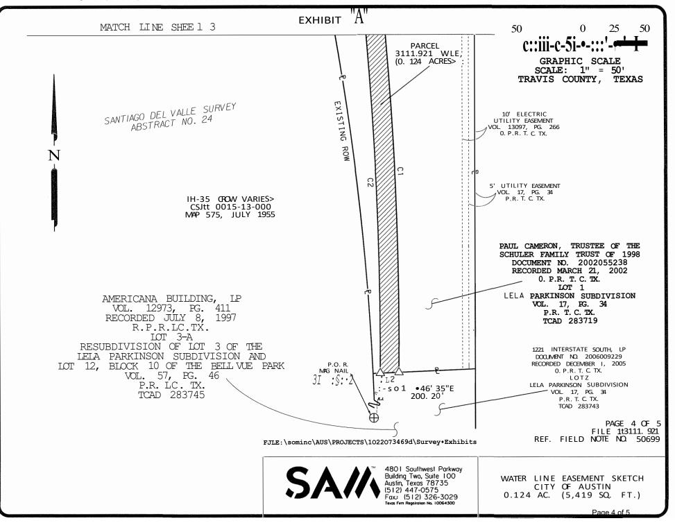
1.ALL BEARINGS SHOWN ARE BASED ON NAD83/2011 TEXAS COORDINATE SYSTEM, CENTRAL ZONE. ALL DISTANCES SHOWN ARE SURFACE AND MAY BE CONVERTED TO GRID BY DIVIDING BY A SURFACE ADJUSTMENT FACTOR OF 1.00011. ALL COORDINATES SHOWN ARE IN SURFACE AND MAY BE CONVERTED TO GRID BY DIVIDING BY THE SAME FACTOR. PROJECT UNITS ARE IN U.S. SURVEY FEET.
