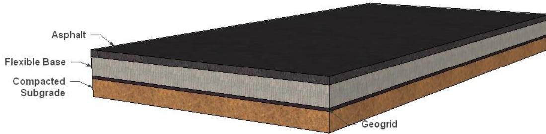
FIGURE 4.2: OPTION 2 FLEXIBLE PAVEMENT TYPICAL SECTION
