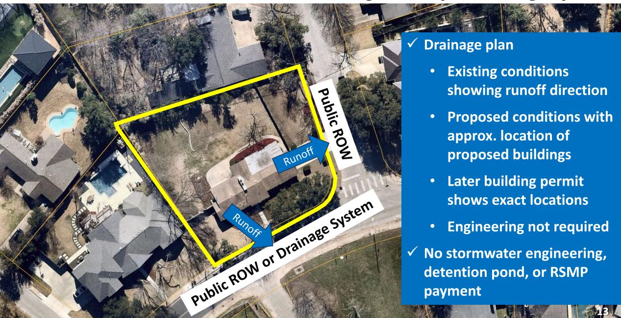
Scenario 2: Lot with surface flows needing to be graded to road/drainage system
