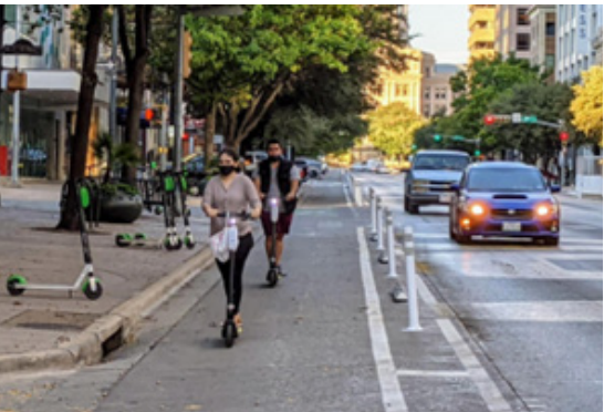
Figure 3.90 - Low-cost, near-term improvements with paint and posts
