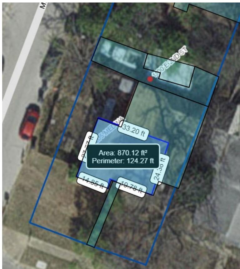
Square footage estimate for portion of property constructed within the period of significance using impervious cover model as baseline ( https://maps.austintexas.gov/GIS/DrainageCharge/ )
