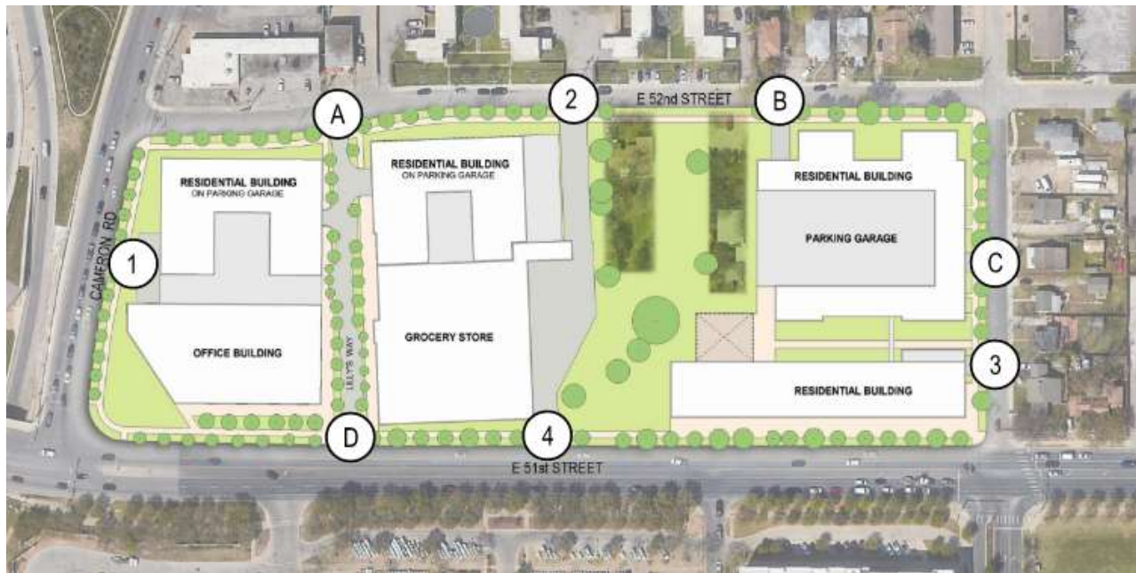
Figure 2. Conceptual Site Driveways (Figure taken from ZTA report); Driveways A, B, C, D are for site access. Driveways 1-4 are service driveways.
